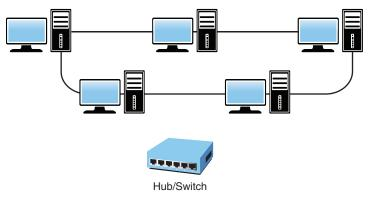
FIGURE 2.5 Logical Design of a Ring Topology
